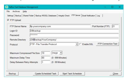
**FTP Upload checkbox:** Select this checkbox if you want to upload files to an FTP site as part of this Backup/Restore job. The checkbox name changes depending on the operation.
